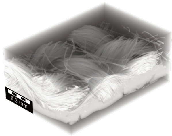
CT scan of PEM fuel cell layer
