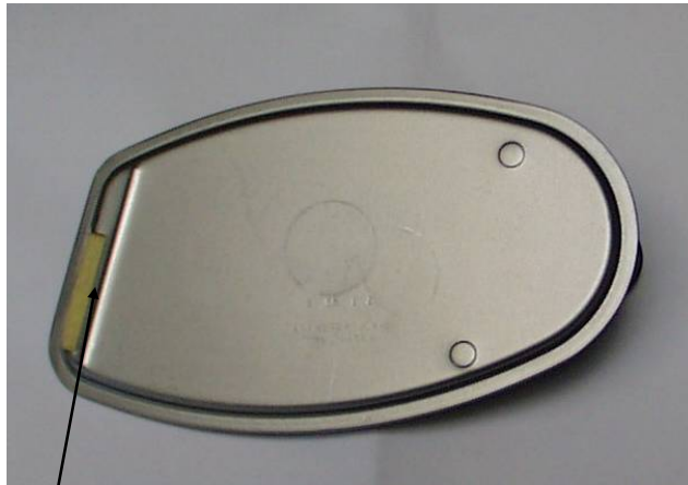
Bottom of suction filter casing
