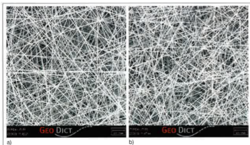
Fig. 3: SEM visualization of 8 volume percent 5 micron fibers at anisotropy 100 (a) and at anisotropy 7 (b), following [5].
