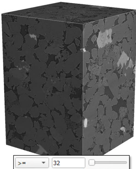
3D gray value representation of a Berea sandstone, showing the entire gray value range.
