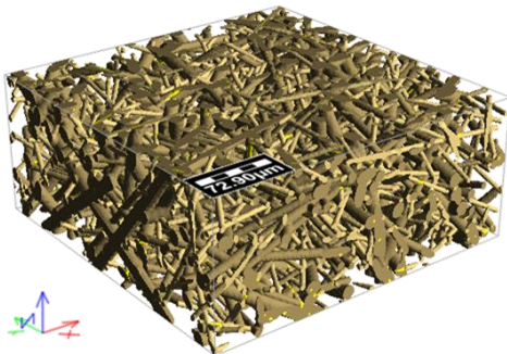
Isotropic fibrous microstructure model generated using FiberGeo
