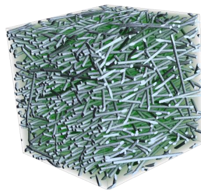
Glass fiber reinforced polymer model generated using FiberGeo
